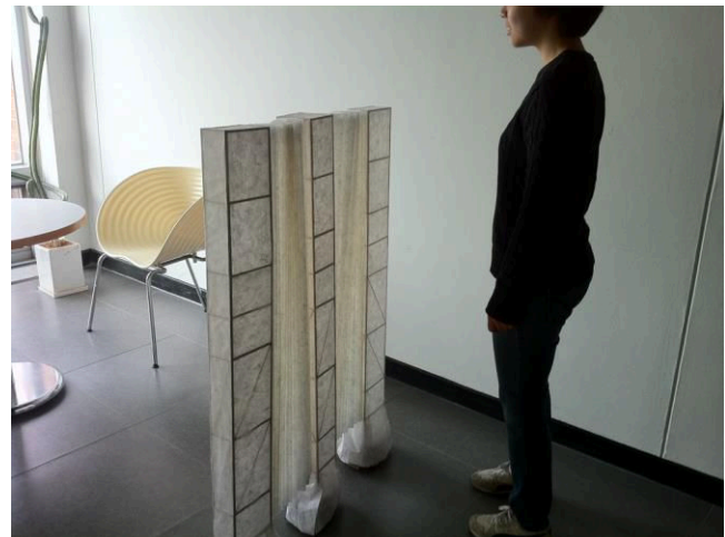
Figure 1. The robotic partition reacting to people around it
